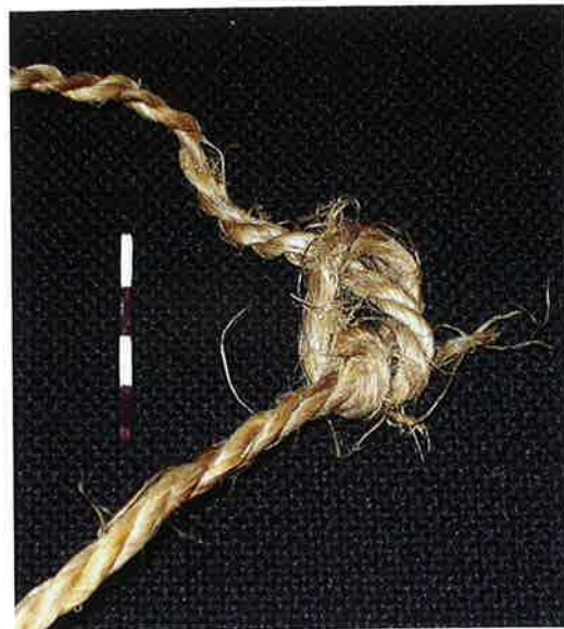
Fig. 9. Condition of the string after 200 shots. – Photo: R. Fontaine.
