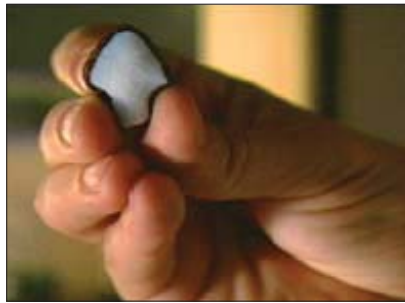
Figure 5. The arrowhead rebuilt by a rapid prototyping process based on three-dimensional tomography CAT-SCAN.
