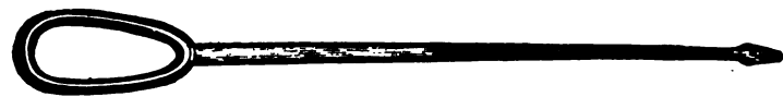
FIG. 35. Wire-twister recommended by Dr. Bill. It should be twelve inches long. (From Dr. Bill's paper.)
