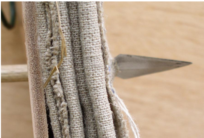
Figure 2. Arrow C shot through one layer of soling leather and 28 layers of linen
