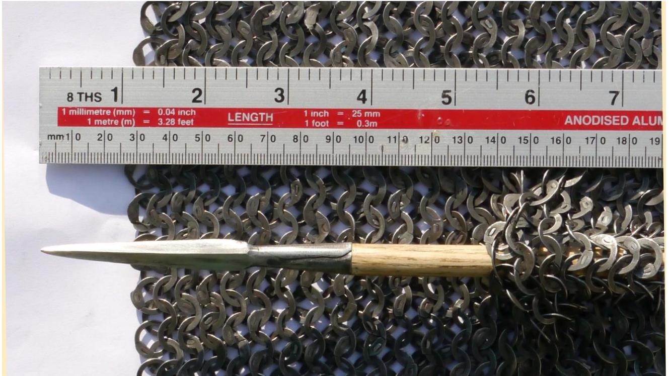
Figure 4. Bodkin Shot through 8 mm Wedge Riveted Mail
