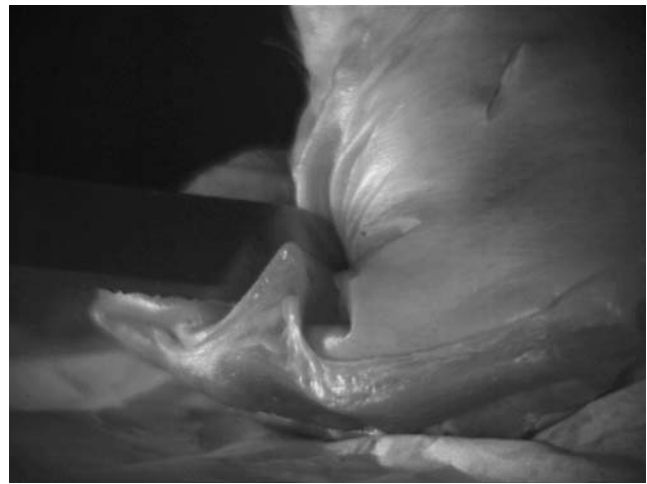
Fig. 13 Gross deflection of the skin without knife penetration at the end of the test with the bread knife
