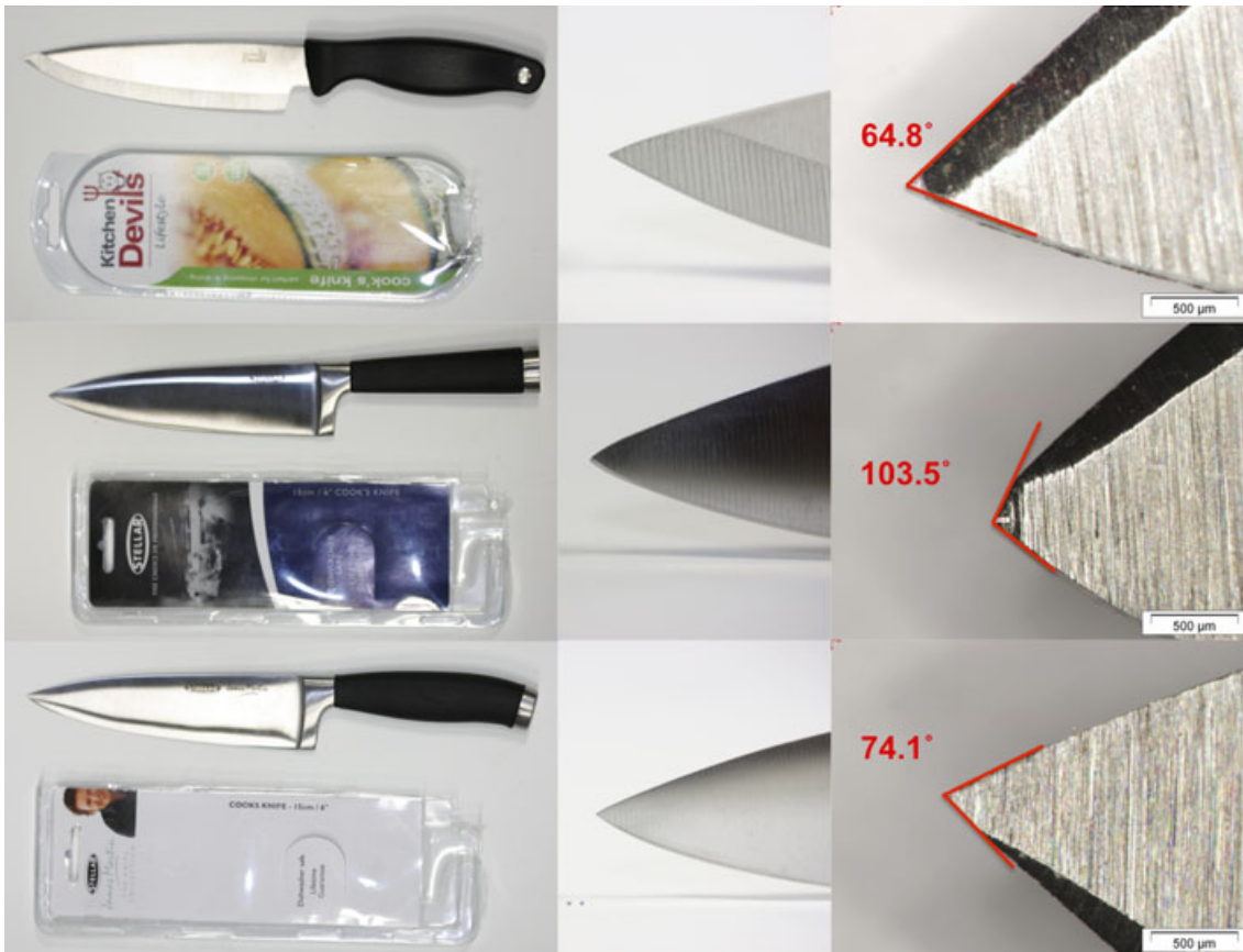
FIG. 8—Composite image showing the three knives used in this study and their tip angles. Kitchen Devil (top) 64.8°, Stellar 1 (middle) 103.5°, and Stellar James Martin (bottom) 74.1°.
